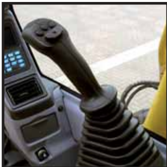
Joysticks with proportional control button for attachments
